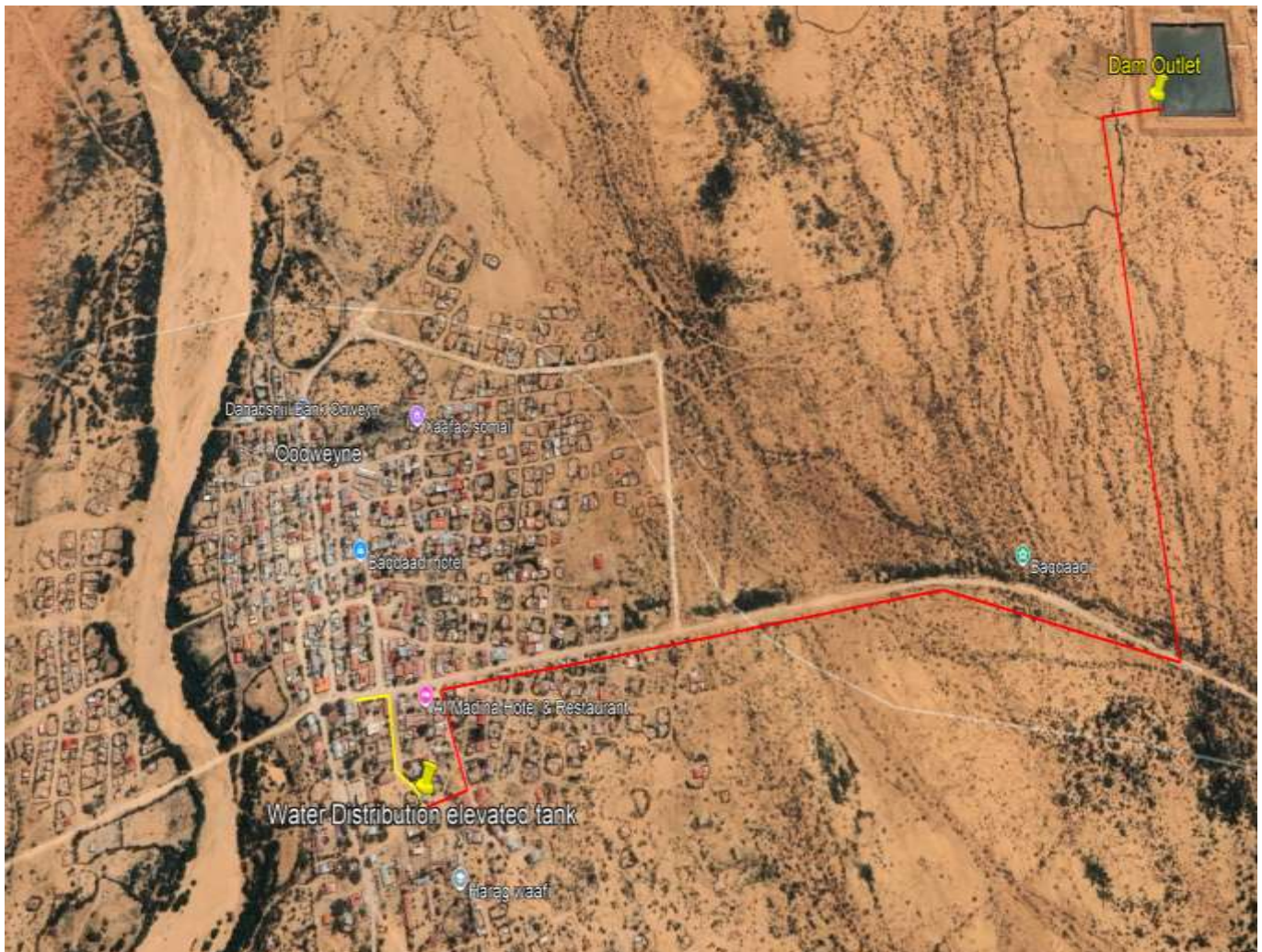
Figure 2 Topographic layout of water supply system
