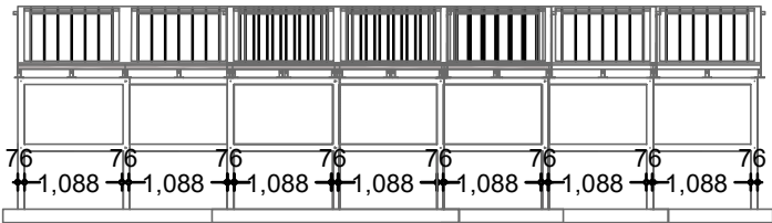
SOLAR STRUCTURE ELEVATION
